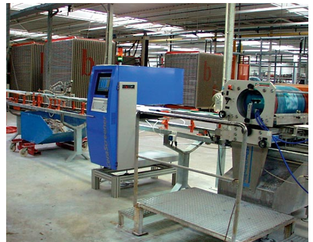
Fig. 4 (bottom) The CeraScreener watches the screen printing process for smallest defects in the decoration by using an advanced colour image comparison technology
