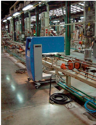
Fig. 8 The stability of the final colour shade is predicted before the tiles are fired using a new colour-camera based vision technology
