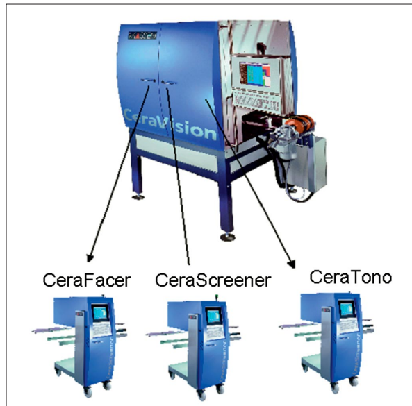
Fig. 1 A family of small, low-cost dedicated vision systems monitoring the tile production before the kiln are derived from the full-blown final automatic sorting system CeraVision
